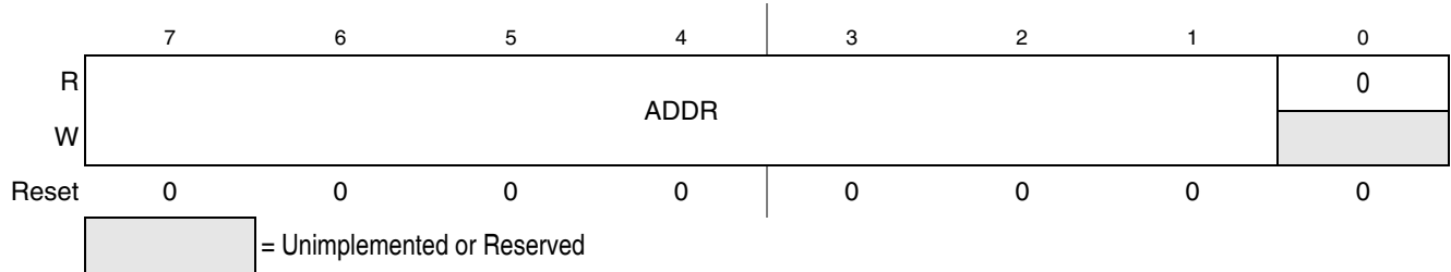
Figure 13-3. IIC Address Register (IIC1A)
