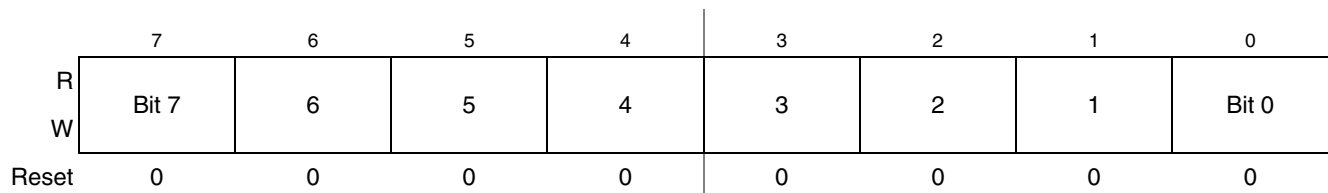
Figure 10-12. Timer Channel Value Register Low (TPMxCnVL)
