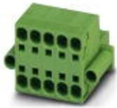
PCB connector, nominal current: 41 A, rated voltage (III/2): 1000 V, number of positions: 4, pitch: 7.62 mm, connection method: Push-in spring connection, color: green, contact surface: Tin
