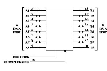
PIN 20=V<sub>CC</sub> PIN 10 = GND
