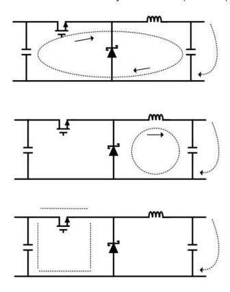
Figure 33. Current Flow in Buck Application
