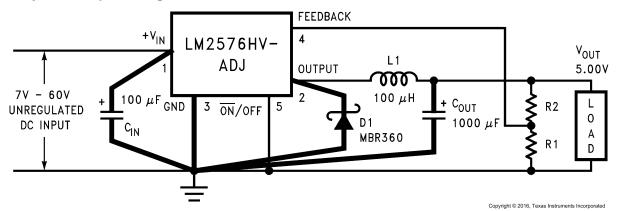
$$\begin{aligned} v_{OUT} &= v_{REF} \left( 1 + \frac{R_2}{R_1} \right) \\ R_2 &= R_1 \left( \frac{v_{OUT}}{v_{REF}} - 1 \right) \end{aligned}$$
