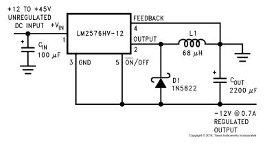
Figure 24. Inverting Buck-Boost Develops -12 V
