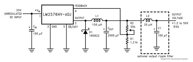
Figure 23. 1.2-V to 55-V Adjustable 3-A Power Supply With Low Output Ripple
