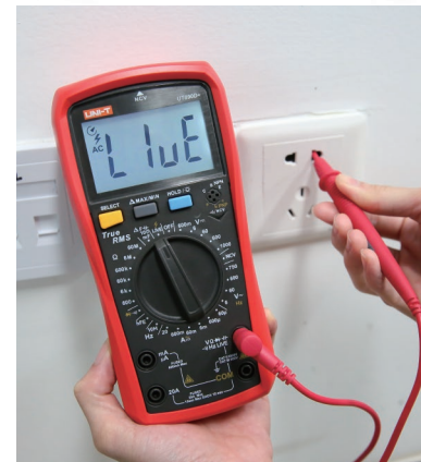
Live and nature wires identification
